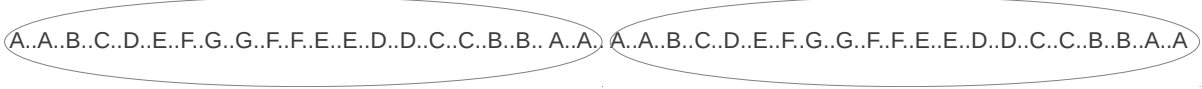
Figure 3.6 Grouping of the communication phases detected for rank 0 of the MG NAS benchmark. The capital letters followed by the double dots represent communication phases followed by interphase gaps, respectively. A single group (shown as solid oval) has been found and the two corresponding subsequences are enclosed into the ovals denoting this group.
